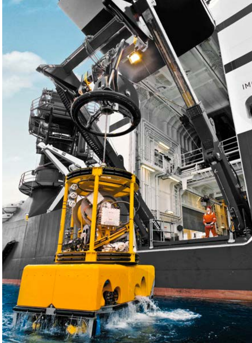
Launch and Recovery System (LARS) of a Remote Operated Vehicle (ROV)
