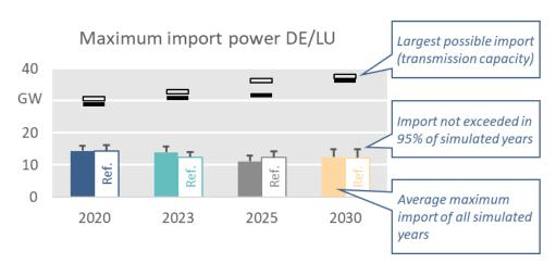
FIGURE 6-13: REQUIRED\* IMPORTS TO DE/LU IN THE "DELAYED NETWORK EXPANSION" SCE-NARIO
