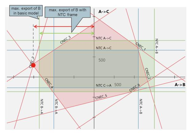
FIGURE B-5: SCALING OF THE FITTED NTCS (GREEN RECTANGLE, "NTC FRAME")
