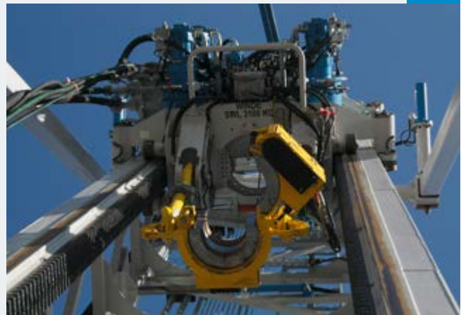
The lifting carriage is moved up and down by remote control.
