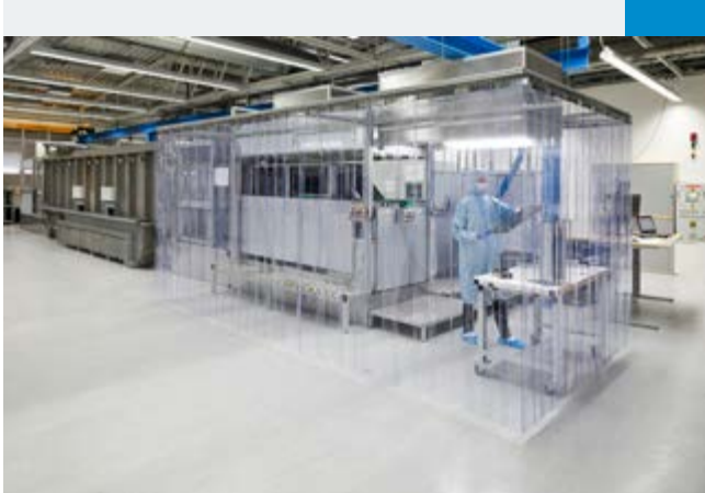
ProConCVD inline epitaxial system in NexWafe technology centre
