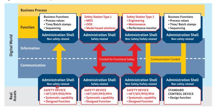
Figure 12 shows an installation of safety-related components in an I4.0 and IM workspace constituting the operational environment within the meaning of IEC TR 63069.
