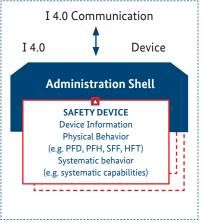
In the event that a safety related device (device with relevance for the safety application) is connected to an I4.0 and IM workspace, it is also attached to an administrative shell. The difference between safety and nonsafety applications is that safety functions
