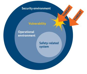
The security countermeasures are defined based on a security risk assessment of the security environment for the SM control system. This is required in order to ensure all relevant security protection targets, Confidentially, Integrity and Availability (CIA), the safety of the system under consideration (I4.0 and IM workspace) and the implemented safety functions.
