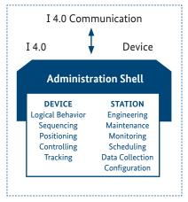
As described above, an I4.0 and IM component in the context of this document is either a device or a station. Each device/station is either equipped with an administration shell. Such an administration shell can either be used to handle an individual
