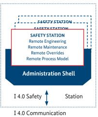
Based on that functionality, safety related devices and safety stations can be allocated in the I4.0 and IM workspace. A safety station is in essence built up following the same concept applied for a safety device too, however a station is con-
